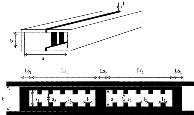
Fig. 1. Layout of the proposed 2 resonator filter.
