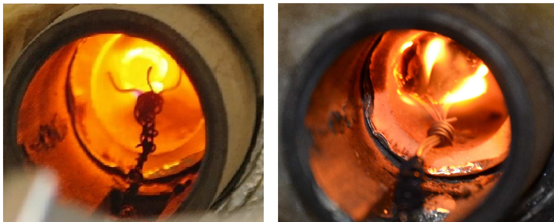
FIGURE B.2: Photos of char (left) and coal (right) particles combustion in GTB
