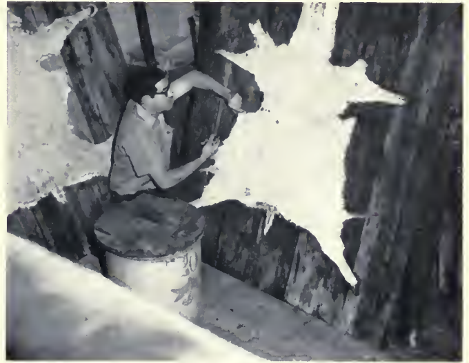
Mario Villa inspects a hide stretched out to dry after completion of the tanning process. Crock in foreground is type used for several soaking processes that skins undergo.
