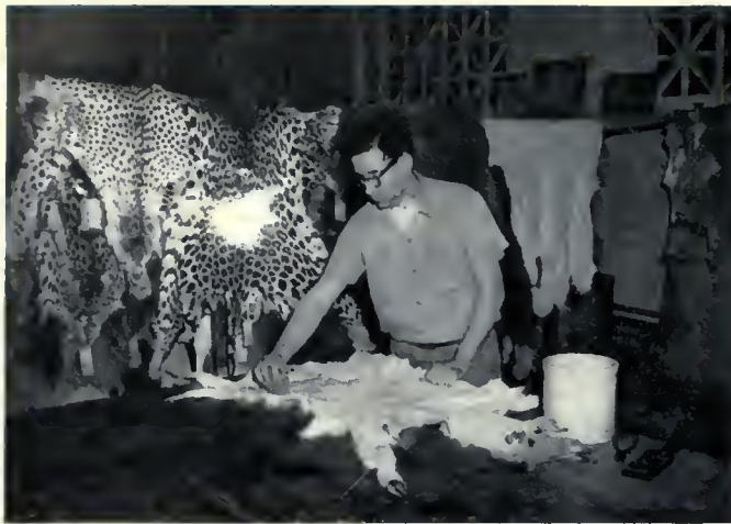
Mario puts the finishing touch on a skin, wetting and shaving it a second time to increase the softness and pliability of the hide.
