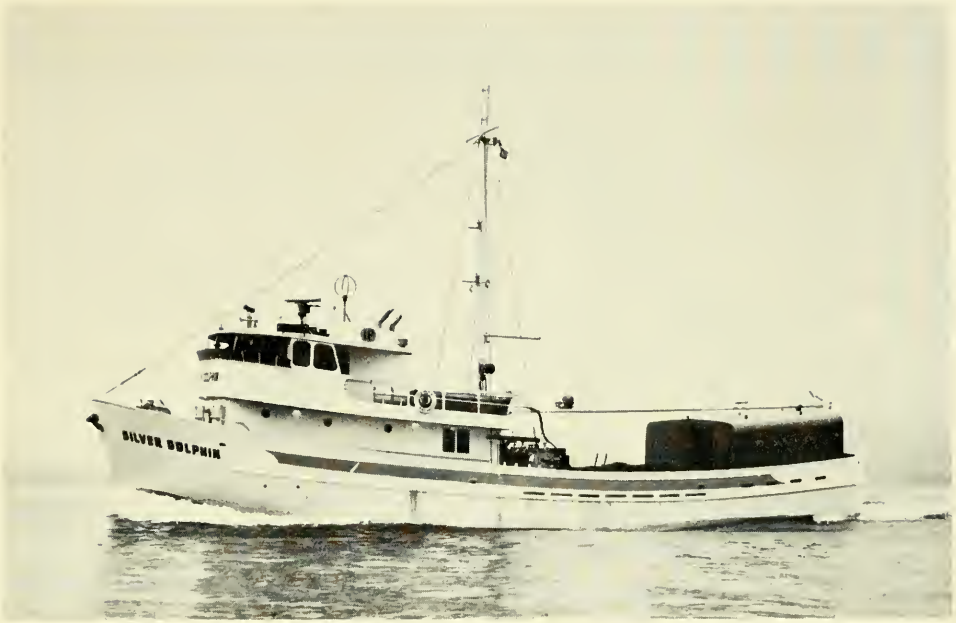
Figure 24. Modern steel seine-boat type "Silver Dolphin" with pilothouse forward and covered baiting and setting area on stern.
