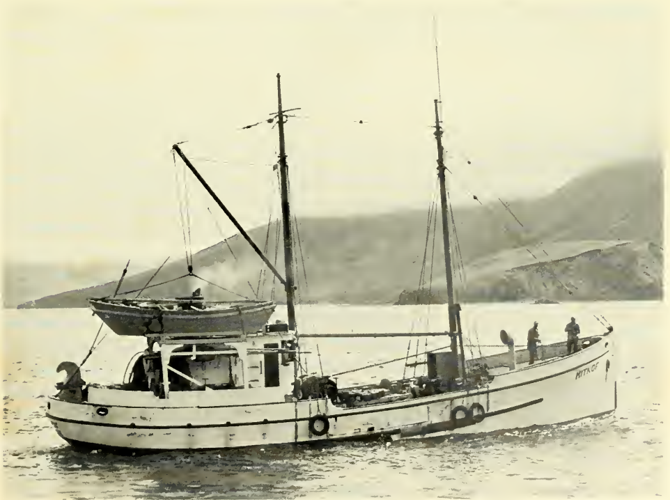
Figure 23. The "Mitkof", a schooner type vessel. Note pilothouse aft and stern chute for setting gear.
