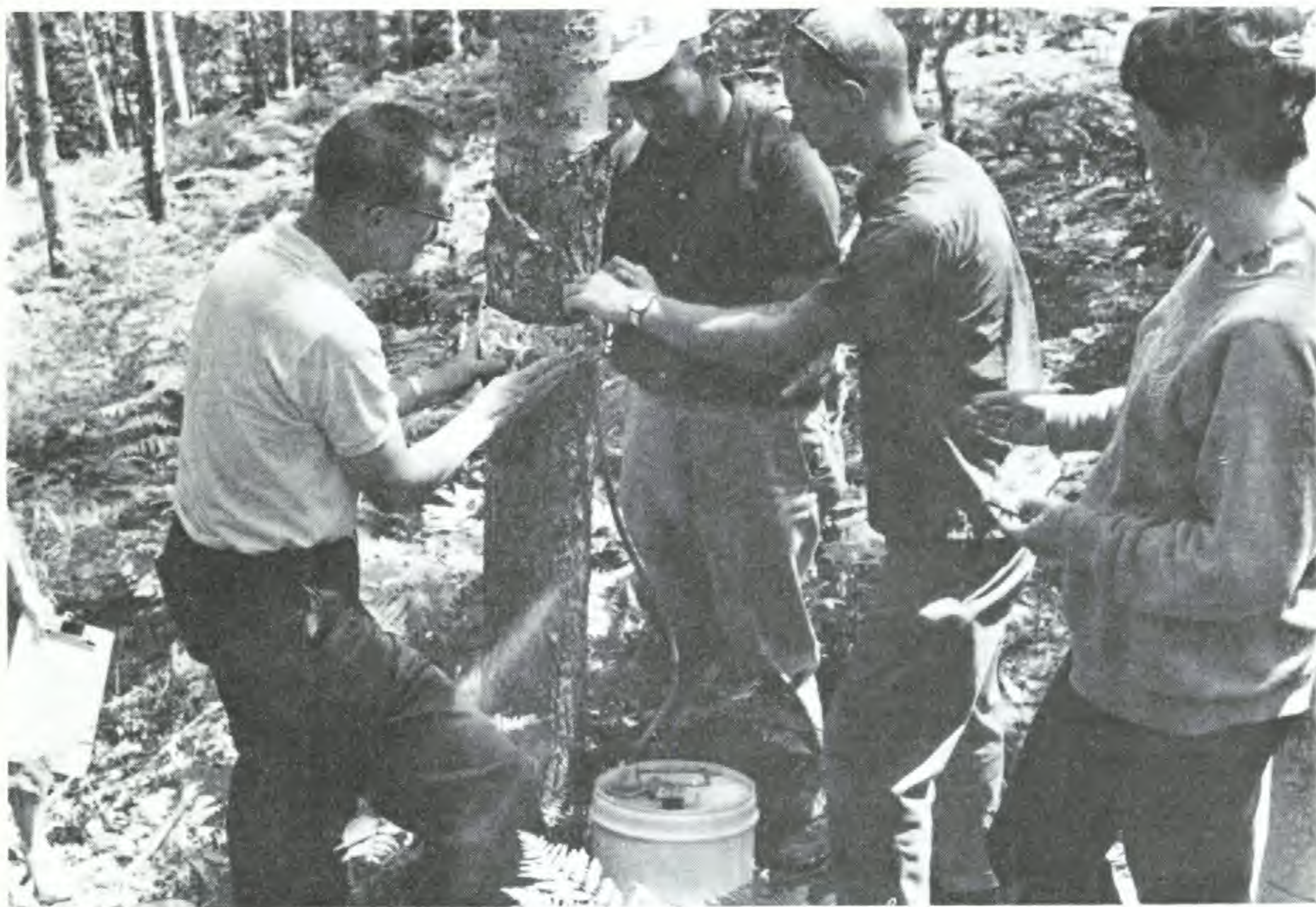
Dr. Gates and graduate students securing a trough and container to measure how much of the rain flows down the trunk. It was 10 times what fell directly!
