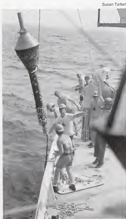
POLYMODE ships were used as ships-of-opportunity to launch free-drifting, satellite-tracked buoys like this spar buoy for studies of Gulf Stream rings.
