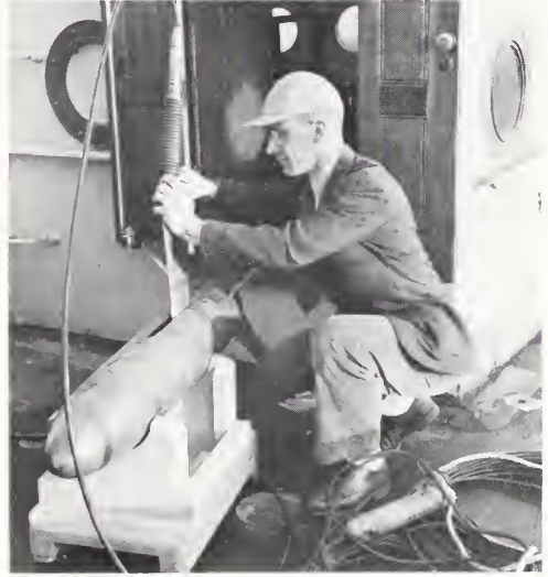
Circa 1948 on the 'Atlantis', Dr. von Arx adjusts a tow fin for the GEK cable and electrodes.
