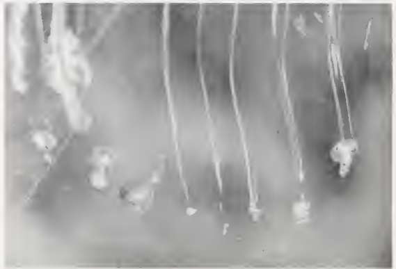
Figure 8. Acrylic dome of the Shark Observation Submersible showing several bite scars (tooth scratches) from attacks by gray reef sharks. (Photos by J. McKibben)
