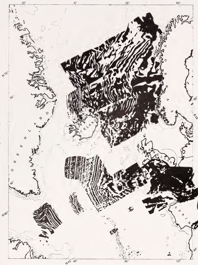
Figure 2: Magnetic anomaly contour chart of the North Atlantic Ocean. The black and white bands portray respectively regions of positive and negative anomalies. Note the obvious symmetrical distribution of banding patterns about the mid-Atlantic ridge crest south and north of Iceland. The thin lines bordering the coastline show the 200-meter and 100-meter bathymetric contour.
