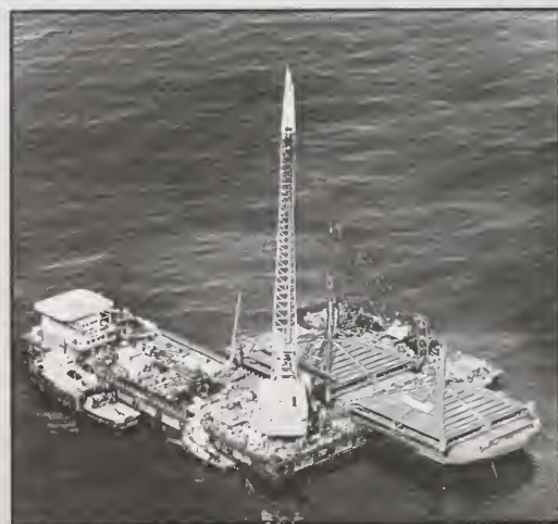
Aerial view of transport barge and marine cranes used by ARCO to carry its two pyramid "caps," now in place over major seeps at Isla Vista, off the Santa Barbara coast. (Photo by Steve Malone/Santa Barbara News Press)
