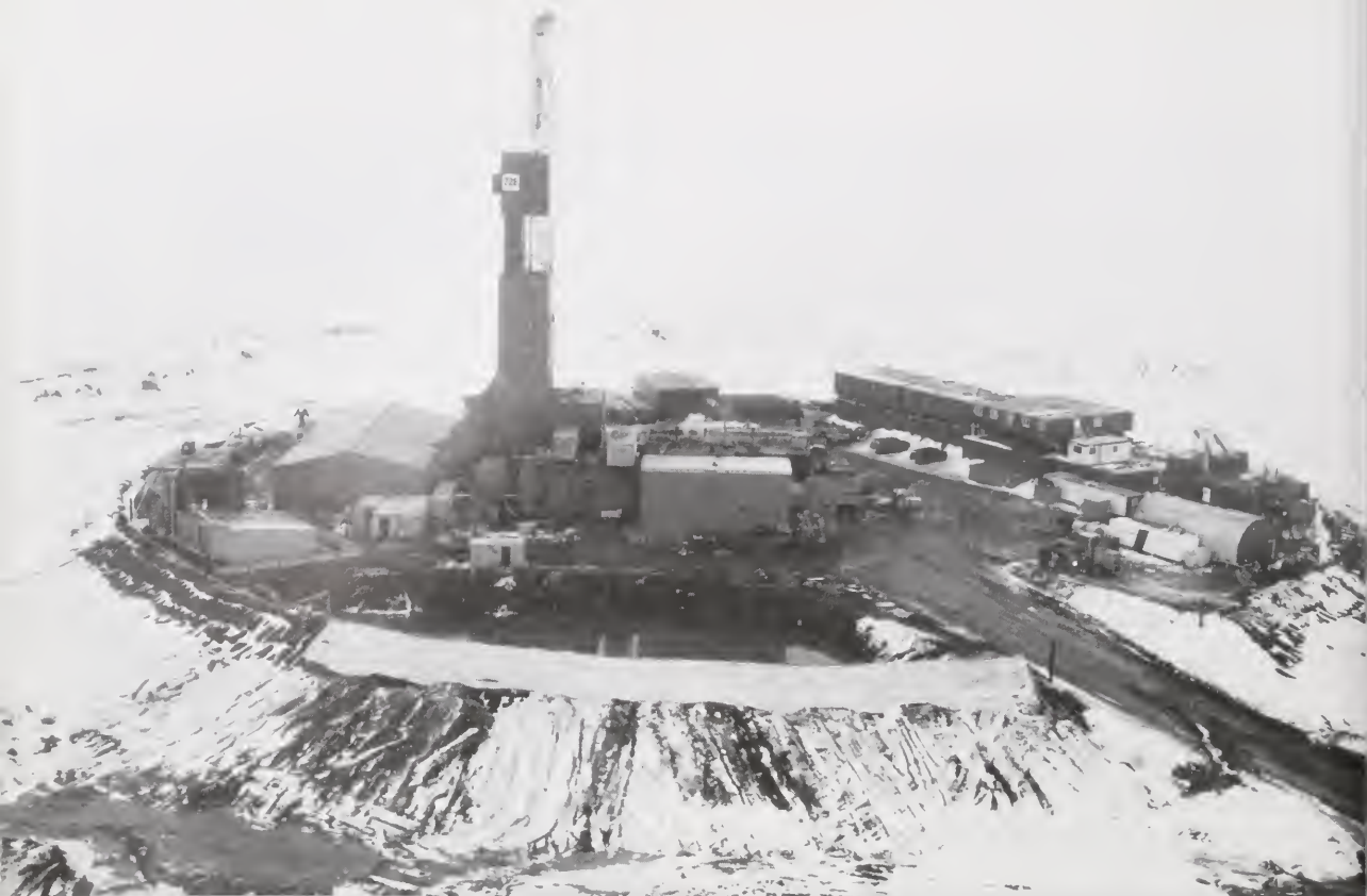
Land rig installed on man-made island in Alaska. (Provided by Petroleum Extension Service, University of Texas at Austin)
