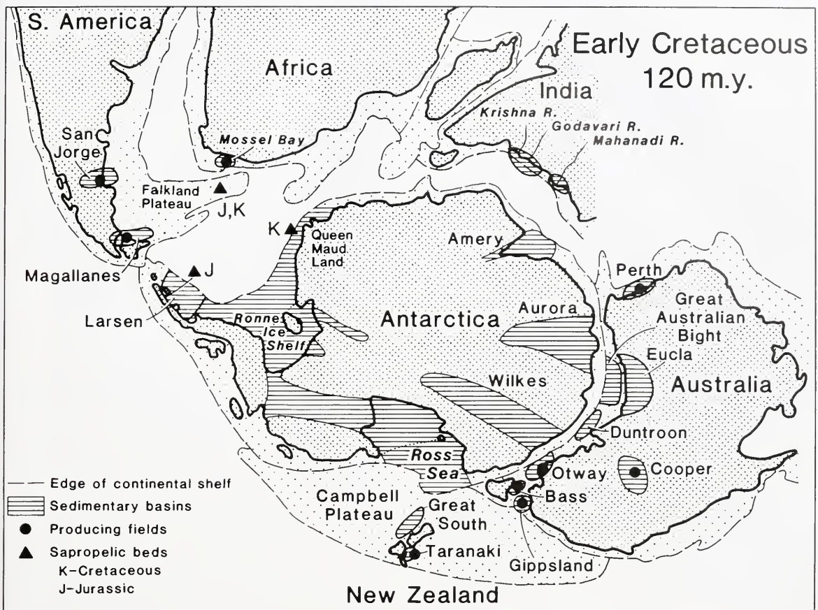
Figure 5. Reconstruction of Gondwanaland in Early Cretaceous time (120 million years ago) shows the proximity of Antarctic basins to basins on formerly adjacent continents, some of which are oil and gas producers. The basins were formed either during the process of rifting of Gondwanaland, or subsequent to that event. The Bass and Otway basins, and that in Mossel Bay, are minor hydrocarbon producers. Subeconomic quantities are present in the Great South Basin and off peninsular India. No hydrocarbons have been reported from the Great Australian Bight, Eucla, or Duntroon basins. It is not clear how many, if any, of the basins on the conjugate margins are analogs for the Antarctic sedimentary basins because of differences in time of formation, sediment thickness, history of deformation, and other factors.
