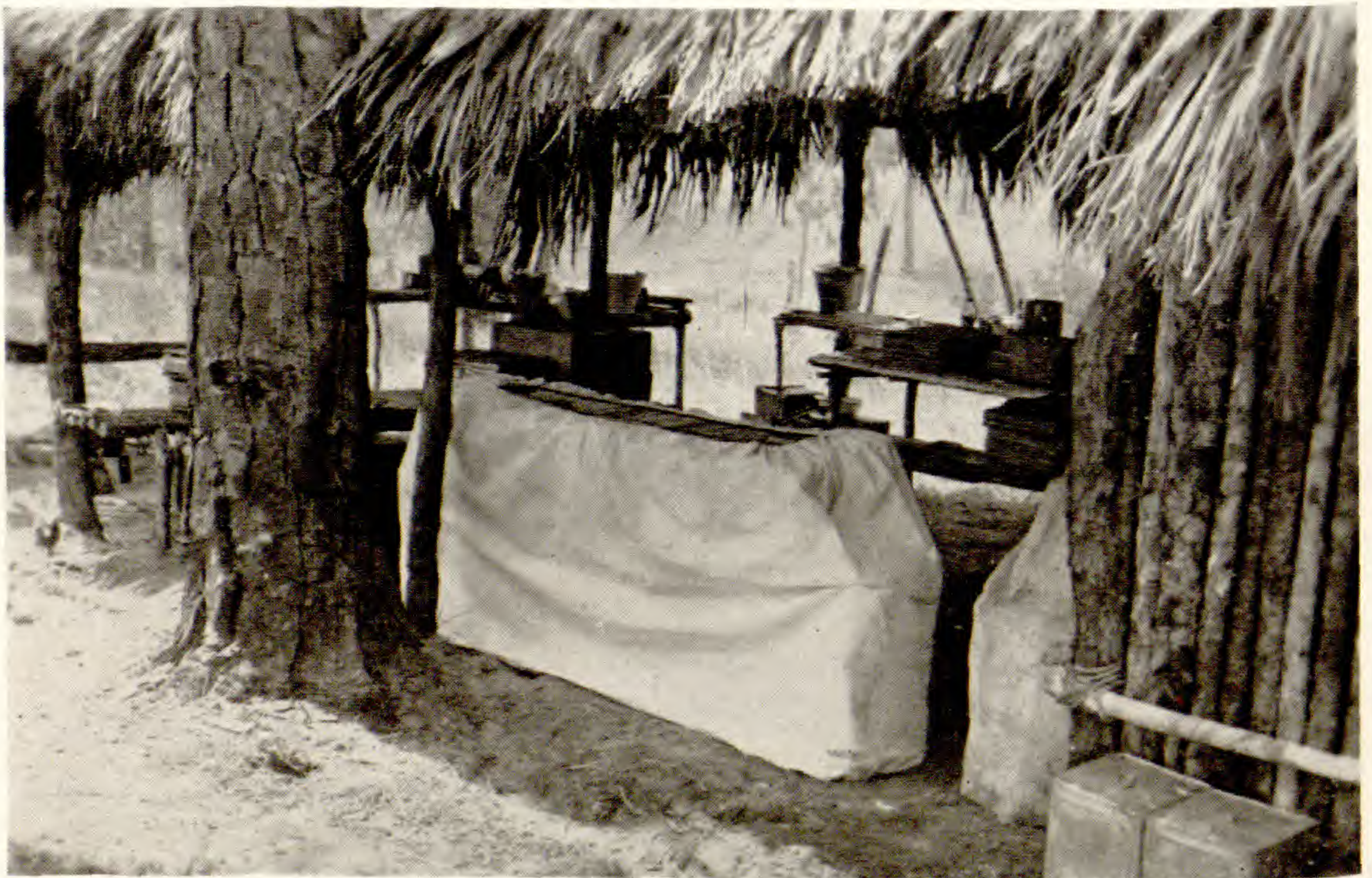
Fig. 5. Plant drier with canvas skirt in place. Note that ample space is left at top to permit the hot air to pass through the corrugated boards.
