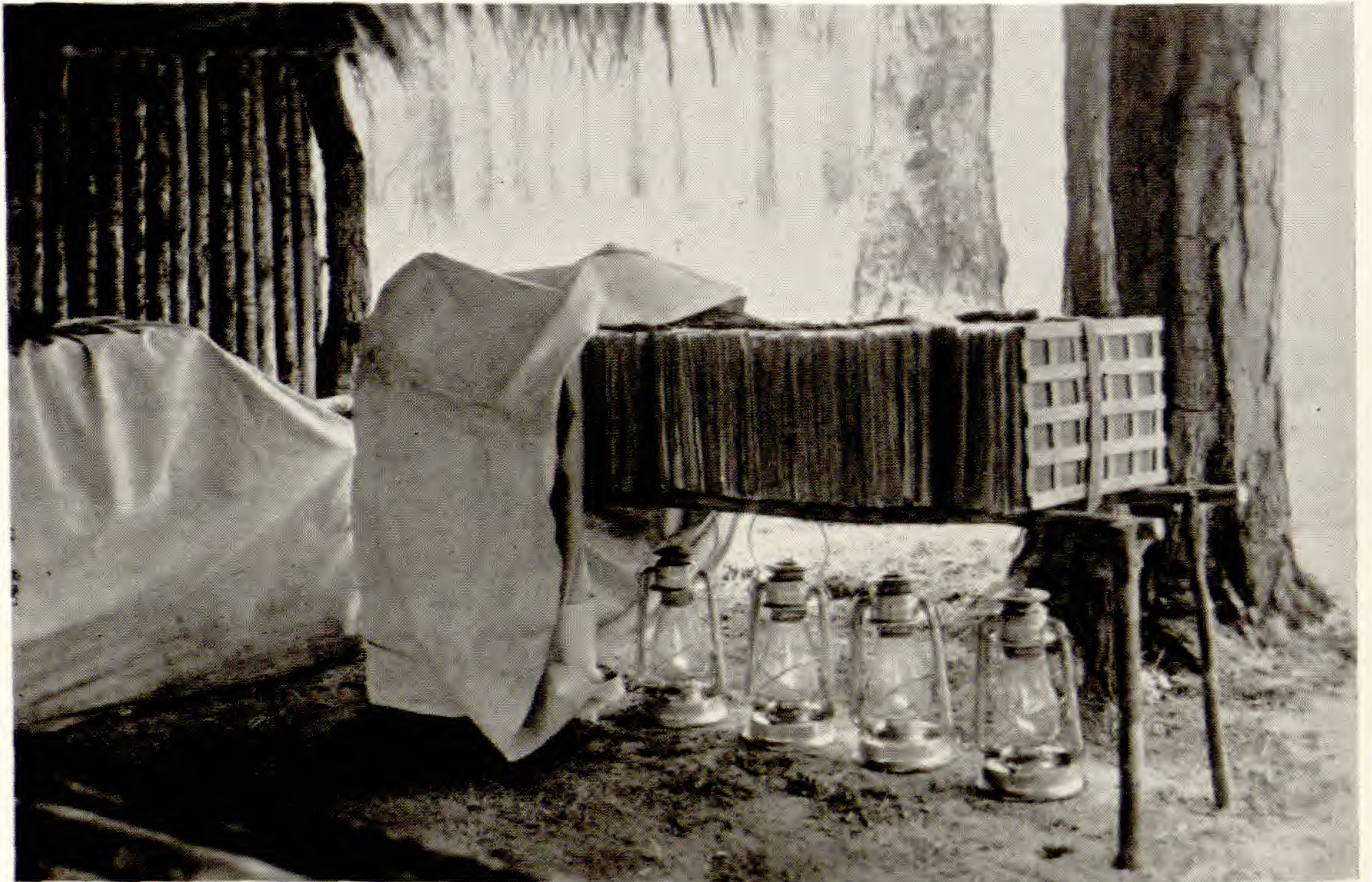
Fig. 4. Plant drier with canvas skirt pulled aside to show presses, frame and lanterns.
