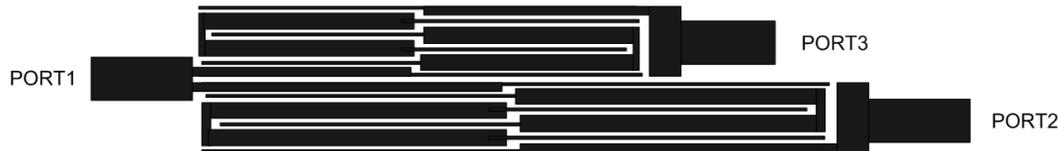
Fig. 4. Layout of proposed microstrip three-port multiplexer
