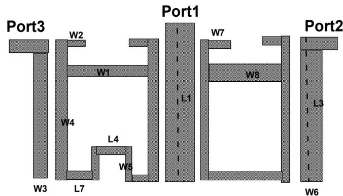
Fig. 3. Layout of proposed microstrip diplexer
