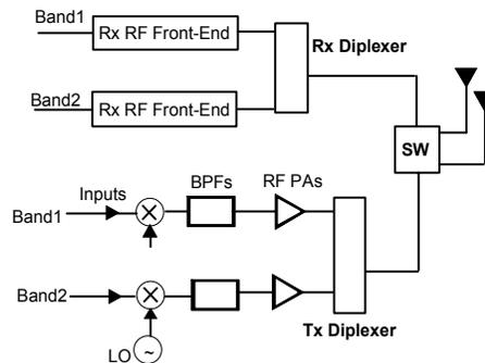
Fig. 1. Traditional structure of WiMAX RF Front-End
