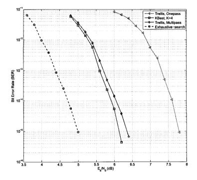
Figure 4.5 Simulation results for a LDPC-coded  $4 \times 4$  4-QAM MIMO system.
