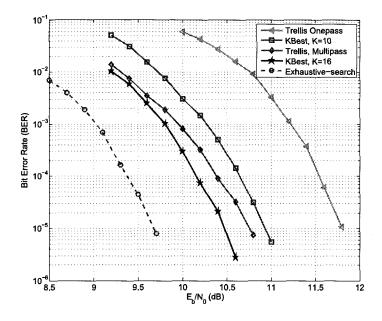
Figure 4.6 Simulation results for a LDPC-coded  $4 \times 4$  16-QAM MIMO system.
