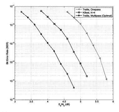
Figure 4.2 Simulation results for a LDPC-coded 2 × 2 4-QAM MIMO system.
