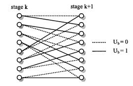
Figure 3.6 3GPP LTE Turbo code trellis with 8 states
