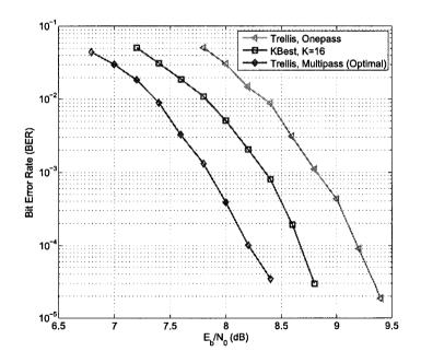
Figure 4.3 Simulation results for a LDPC-coded  $2 \times 2$  16-QAM MIMO system.
