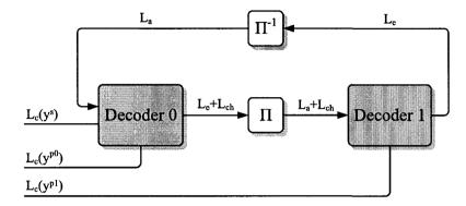
Figure 3.5 Overview of Turbo decoding
