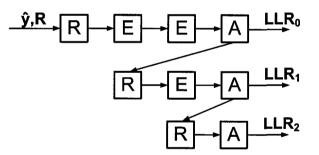
Figure 4.1 CUDA MIMO detector data flow
