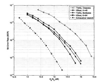
Figure 4.7 Simulation results for a LDPC-coded 4 × 4 64-QAM MIMO system.
