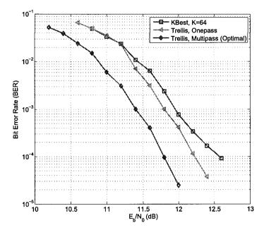
Figure 4.4 Simulation results for a LDPC-coded  $2 \times 2$  64-QAM MIMO system.
