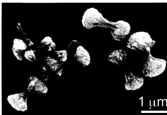
Figure 2.12. SEM image of iron phosphide nanorods synthesized with the addition of 100 \mu\text{L} hexane.
