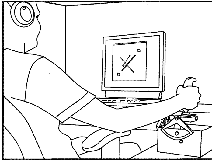
Figure 5.1 : A participant is sitting at the virtual training environment. The interface includes a visual feedback display and a haptic joystick for force feedback. The training task is shown on the visual display with the visual guidance activated.
