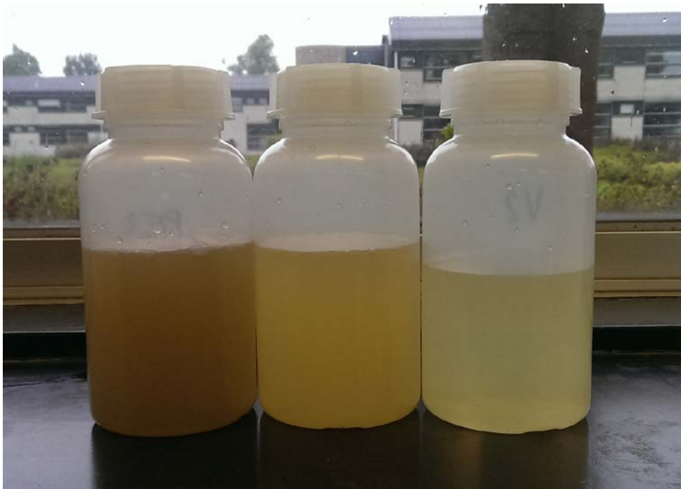
Figure 1 The fluids after extraction (left), after 12-40 \mu\text{m} (middle) and after 0.6 \mu\text{m} (right) clarification steps
