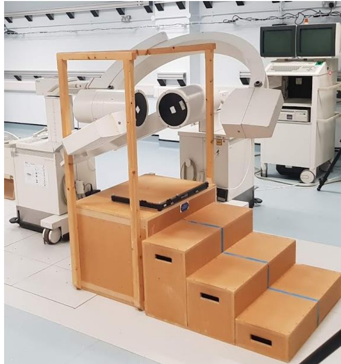
Figure 6-1 Adapted stair set with two C-arms positioned to allow investigation of tibiofemoral kinematics during a stair activity.
