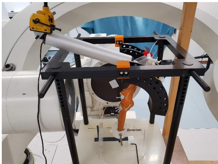
Figure 5-24 Linear actor mounted to the top of the custom knee rig connected to the proximal end of the femur in the middle of the C-arms field of view. The c-shape runners were used to direct the travel of the linear actuator and the distal end of the tibia was clamped to the base of the rig to ensure the phantom remained in the field of view of the X-ray equipment.
