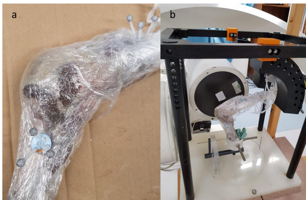
Figure 5-25 a Ovine specimen with marker clusters implanted into tibia and femur; b Ovine specimen fixed into the custom knee rig in a static position.
