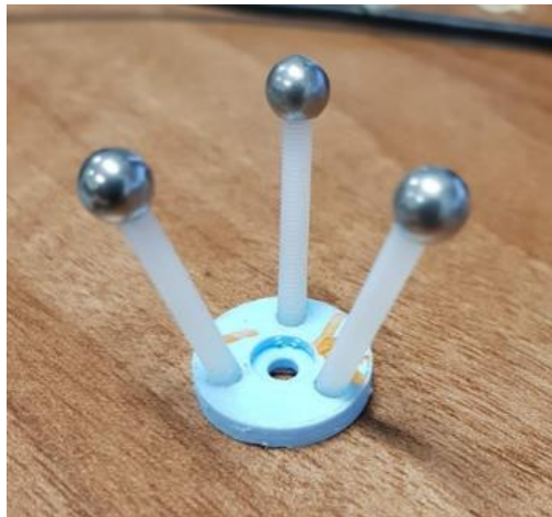
Figure 5-20 Custom marker cluster holding three 6mm stainless steel balls
