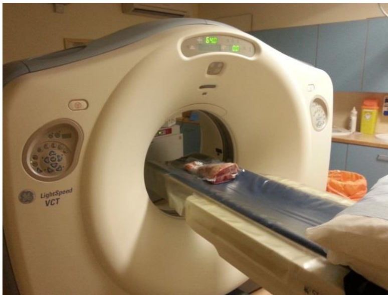
Figure 4-7 Ovine specimen being CT scanned by a GE Lightspeed VCT scanner
