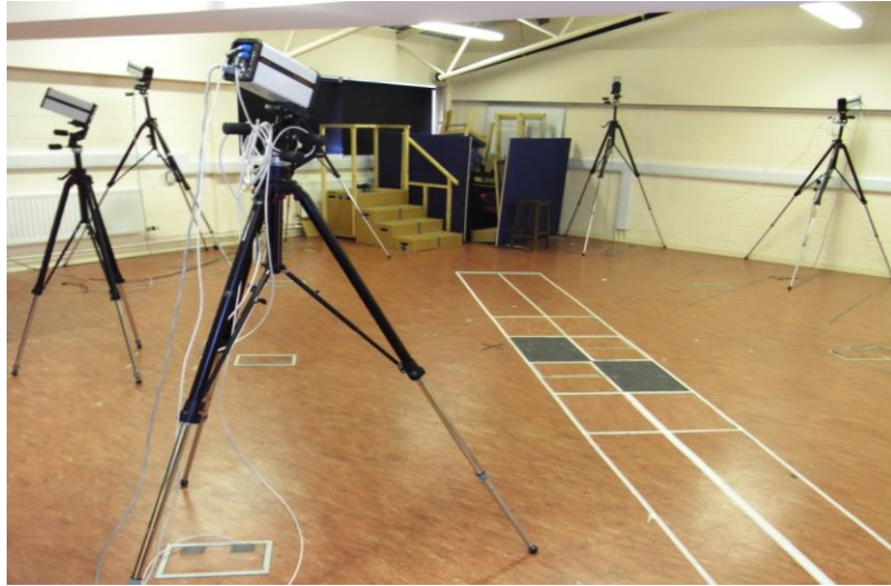
Figure 2-1 Pro reflex cameras and patient walkway fitted with force platforms in the Cardiff Motion Analysis Laboratory
