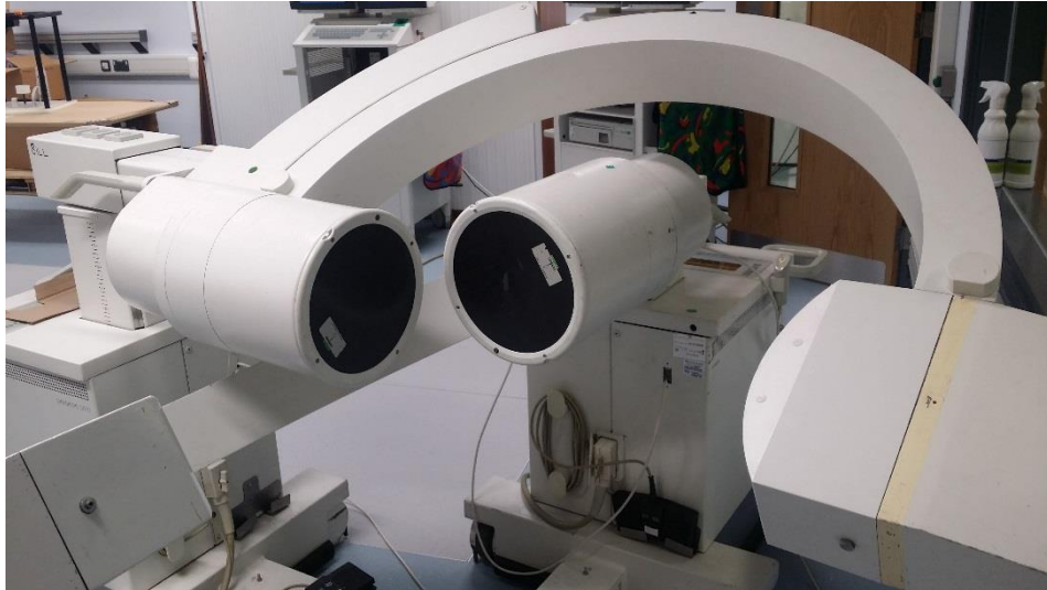
Figure 5-2 Final configuration of the two C-arms that was used for all experiments in Chapter 5 and Chapter 6. The angle between the two imaging fields was approximately 90^\circ . The C-arms were rotated axially to 60^\circ and 120^\circ respectively to allow overlapping field of views. The cameras inside the C-arms were rotated to correct for the axial rotation applied to each C-arm.
