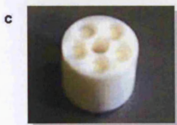
Fig. 1.12 a) The Constant Depth Film Fermenter (CDFF); b) close up of the rotating turntable; c) PTFE pan with 5 recessed plugs; d) close-up of the scraper blade
