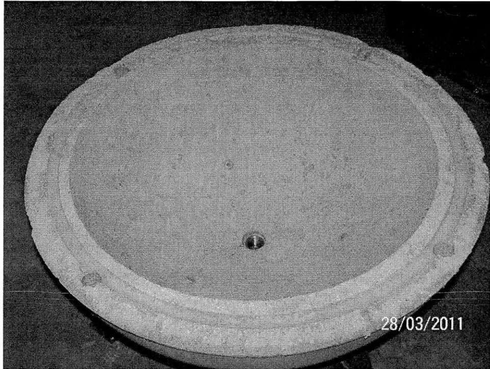
Figure 12 A concrete hemisphere fresh out of the mold. The pipe coupling can be seen embedded in the pole.
