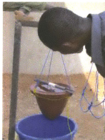
Figure 64: Flow rate testing (Source: Bradner)
