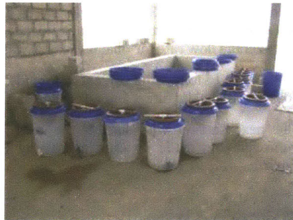
Figure 61: Filter flow rate tests
