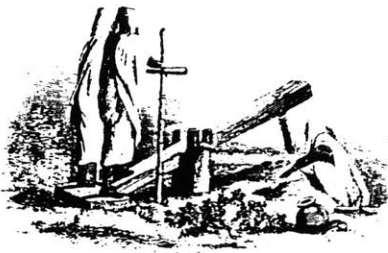
Fig. 3.2.6 Dheki is the apparatus used for husking rice
