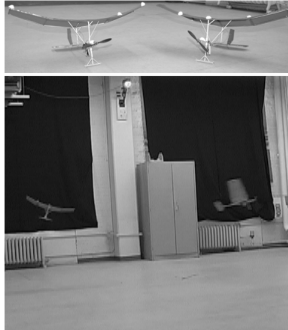
Figure 15. Above: Micro-UAS designed for Real-time indoor Autonomous Vehicle test Environment (RAVEN). Below: Micro-UAs engaged in Basic Fighter Maneuvering (BFM) during flight test.
