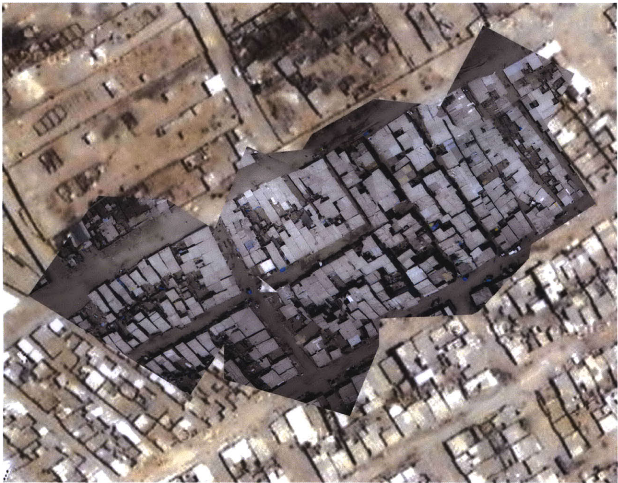
Figure 7.4: Completed balloon map of Juan Pablo II, produced with Adobe Photoshop CS4. The map is overlaid on imagery from Google Maps for comparison.
