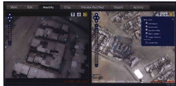
Figure 7.7: Demonstration of JavaScript hack to insert Google satellite data for warping in areas with low feature density. [82]
