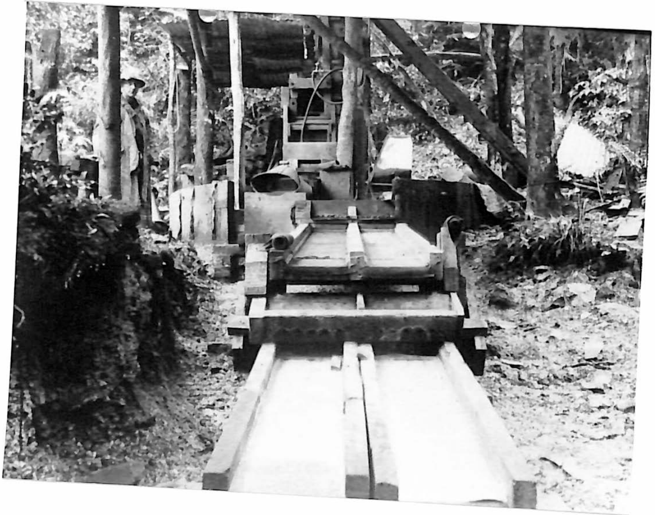
Figure 22: Riffles in Malcolm Hardy's plant, 1930s, David Calder Hardy Collection; used with permission,
