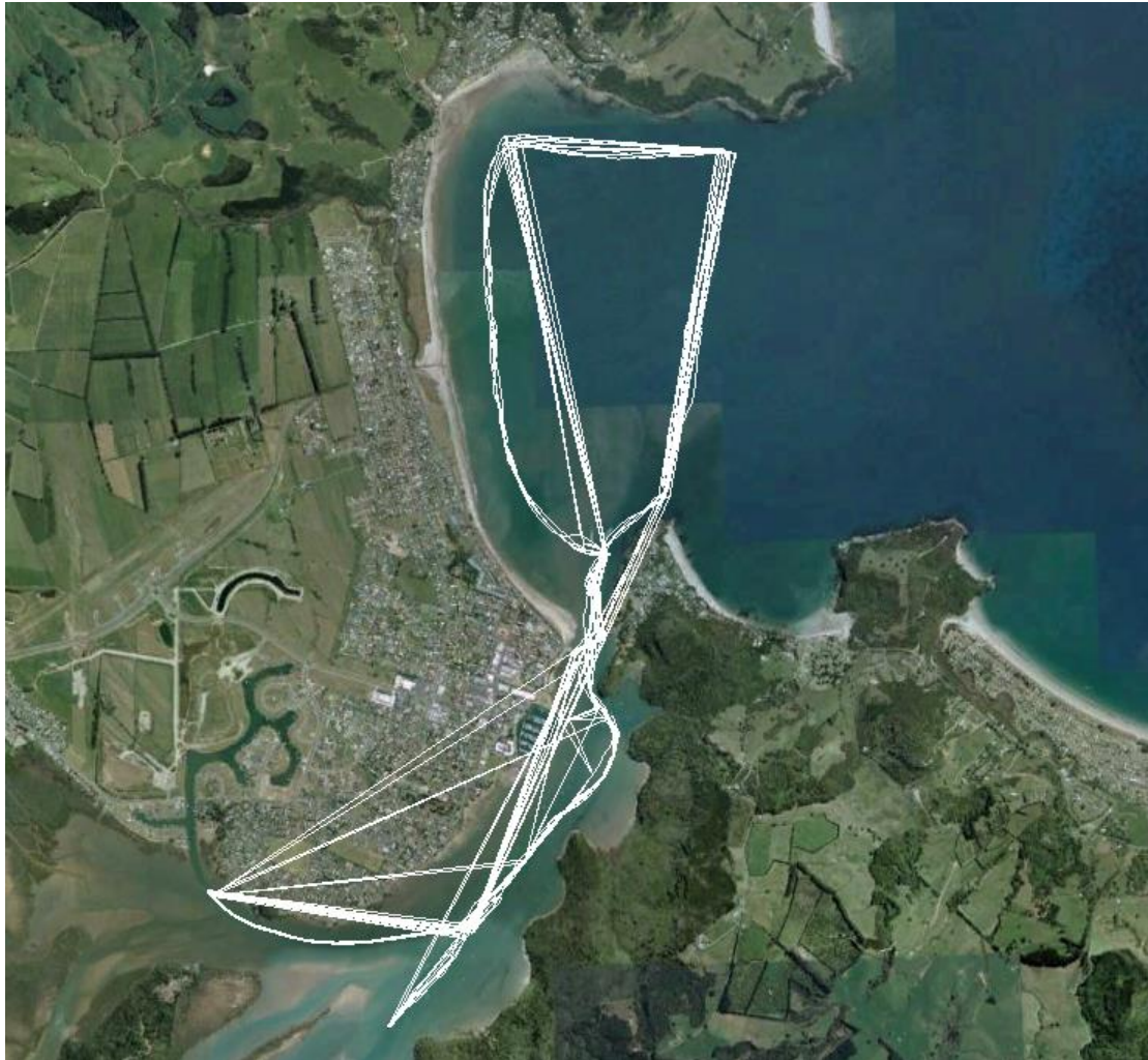
Figure 12 - ADCP current survey GPS path encompassing an entire spring tidal cycle taken over the span of 2 days during the 2015 deployment.
