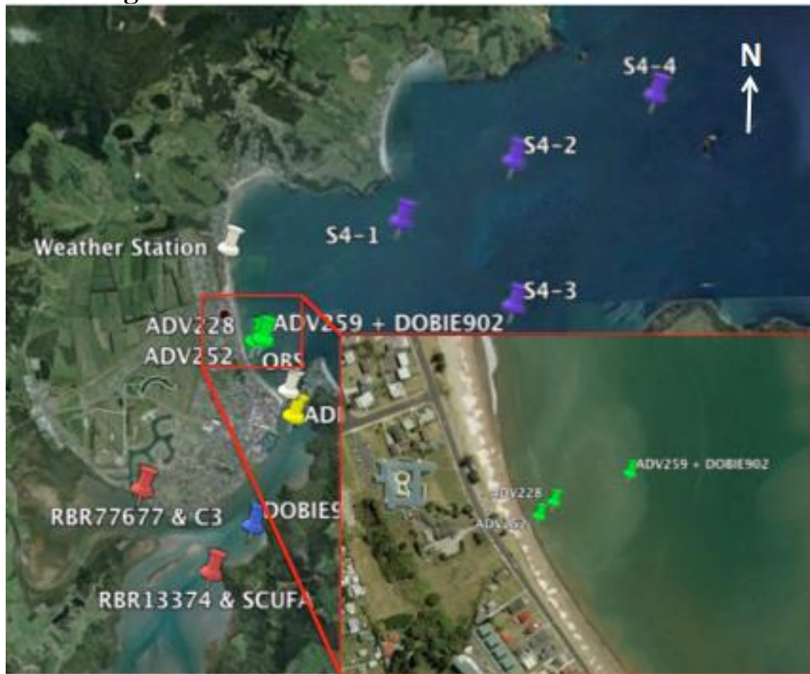
Figure 3 - The ADVs were moved from a shore parallel configuration to a shore normal transect. DOBIE 911 and DOBIE 802 were retrieved. All other instruments remained unchanged. (Imagery: Google Earth).
