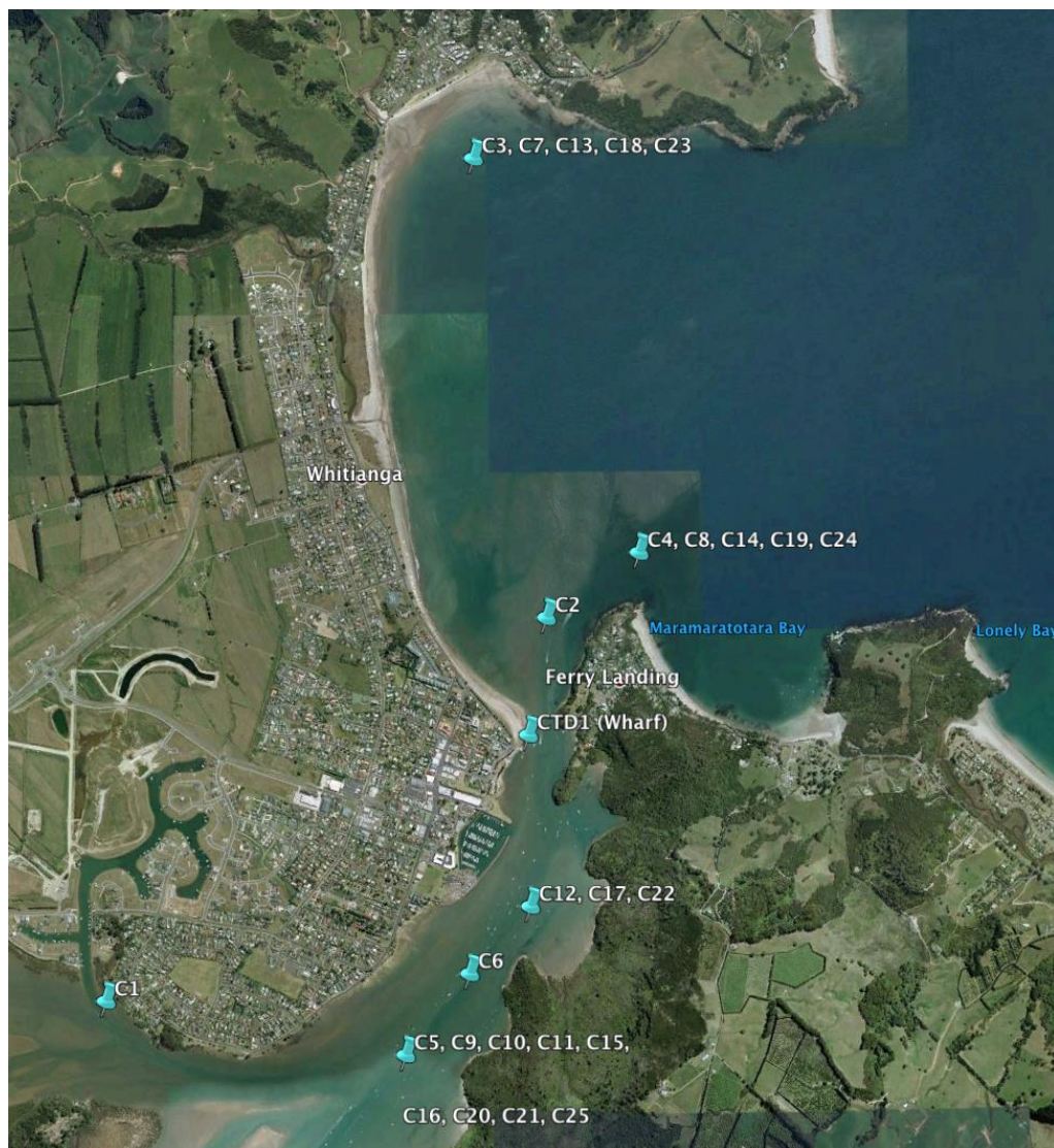
Figure 15 - CTD casts taken at the wharf (CTD1) and within the estuary/bay simultaneously with CTD2 aboard R/V Taitimu. (Imagery: Google Earth).
