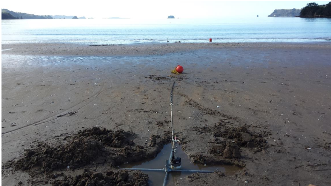
Figure 4 - ADVs in a shore normal array buried on the beach (July 24 th , 2014). ADV order from foreground to background: ADV252, ADV228, and ADV259 & DOBIE902 (submerged – marked by buoy). ADV252 and ADV228 cycled between submerged and exposed with the tide.
