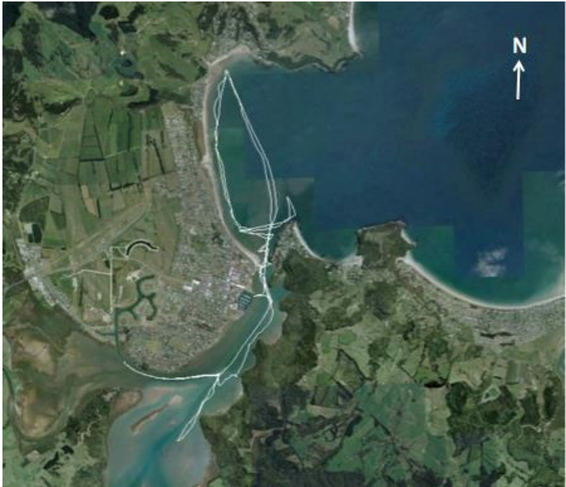
Figure 10 - ADCP current survey during incoming tide and slack water. (Imagery: Google Earth).
