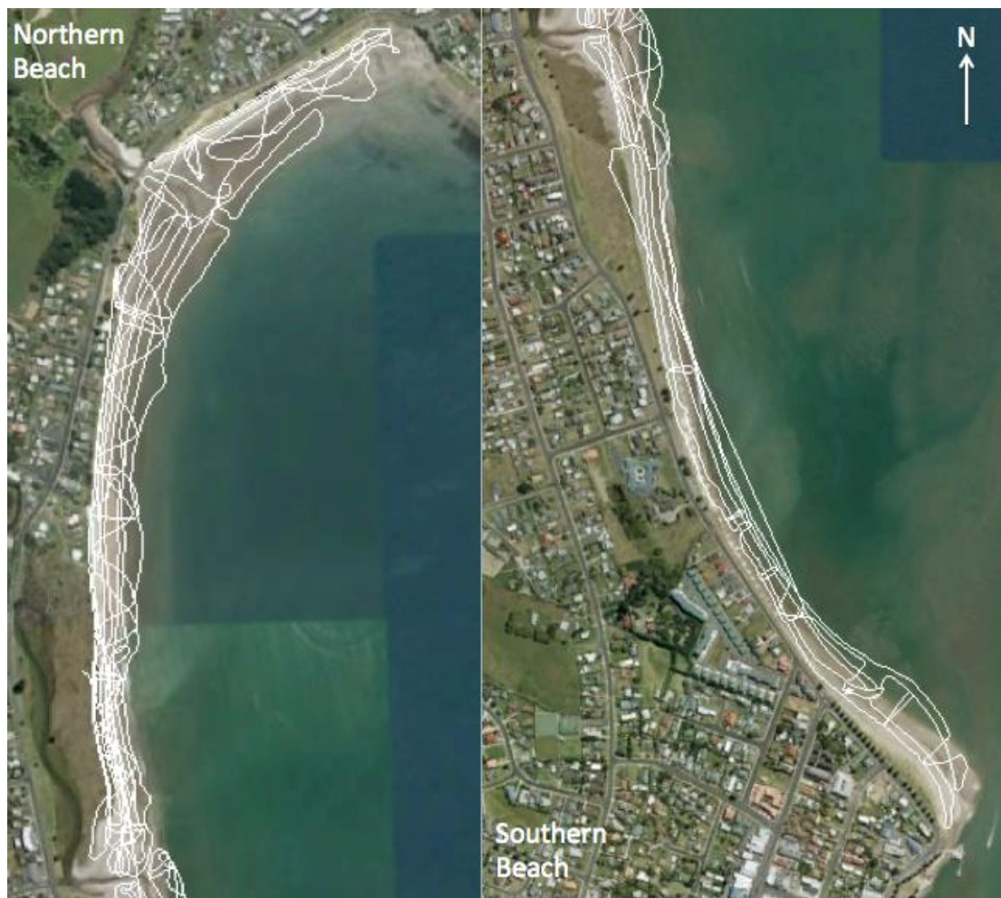
Figure 13 - Buffalo Beach RTK GPS survey during low tide on 23/7/2014. GPS receiver was mounted to a quad bike. (Imagery: Google Earth).
