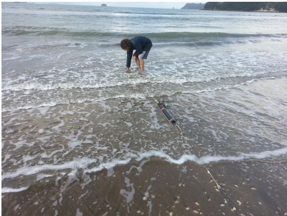
Figure 9 - Ben Stewart securing a Nortek Vector with anchors into the surf zone on May 7 th , 2015. The instrument recorded two full tidal cycles before being removed on May 8 th , 2015.
