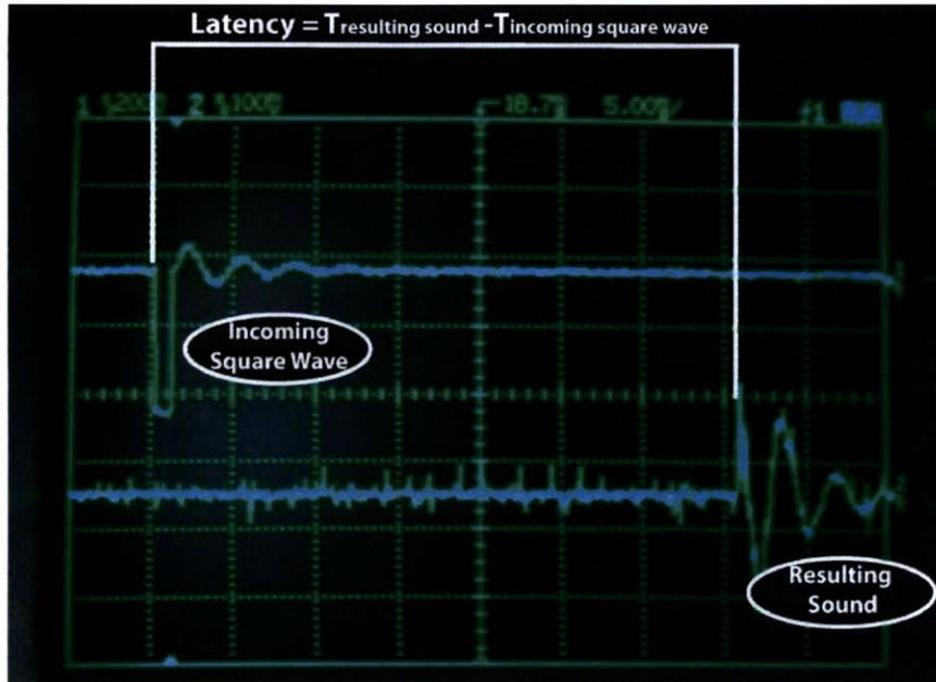
microphone. The o-scope was then used to measure the shift from the incoming square at the microphone to the outgoing square leaving the iPaq. Ssee figure 9.
