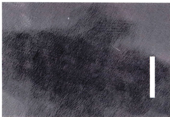
Figure 3.8 a) Proposed route towards molecular wires composed of a string of individual single-molecule magnets with aligned crystalline axes. b) TEM micrograph of molecular wires (7) . Scale bar = 10nm.
