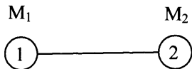
Figure 2-28: Nodes with disjoint information. Node i has M_i disjoint data packets (or independent random linear combinations of packets). Both nodes want to have all the information at the end of the exchange.
