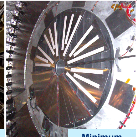
Minimum Bias Trigger Scintillator
