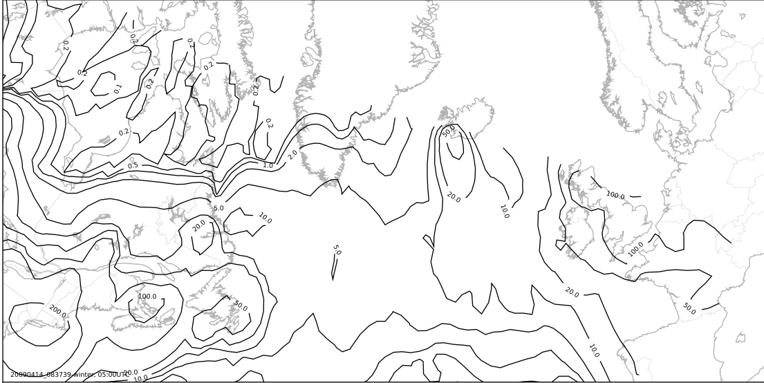
Figure 4-4: Downlink capacity contour plot for winter data set at 5:00UTC. Averaged over all simulation runs. Capacity measured in Mbps.
