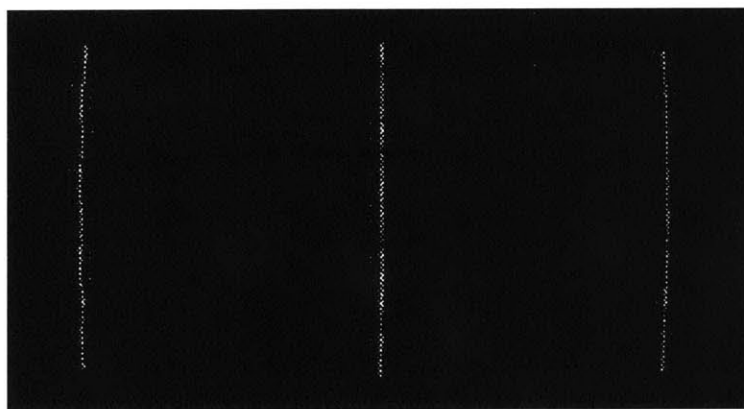
Figure 6.6 Test pattern consisting of one central vertical line and two lines at the edge of the field. The lines are image 3 mm from the Bragg cell plane.
