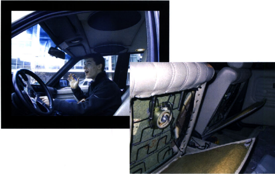
Figure 5.7: Two small parametric arrays were mounted overhead in this automobile experiment, and subwoofers were embedded directly within the seats. It was found that the low-frequencies were effectively heard by the intended listener, but were not noticeable by the other passenger.
