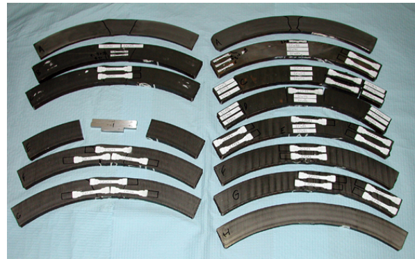
Figure 3. Shows the preparation of test specimens from each weldment, TB repair weld LHS and fabrication weld RHS.
