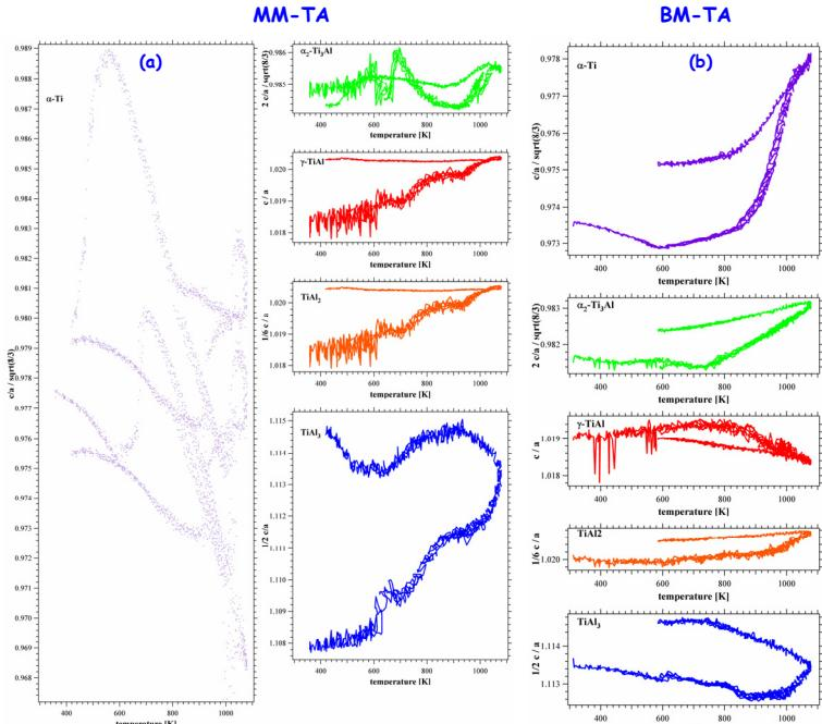
a and b: Lattice parameter ratios c/a normalized to closed packed ratios as a function of temperature for MM-TA and BM-TA, respectively.
