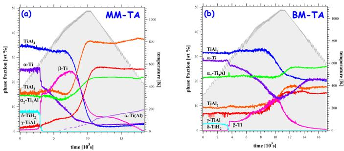
a and b: evolution of phase fractions obtained by Rietveld refinement as a function of temperature for MM-TA and BM-TA, respectively.
