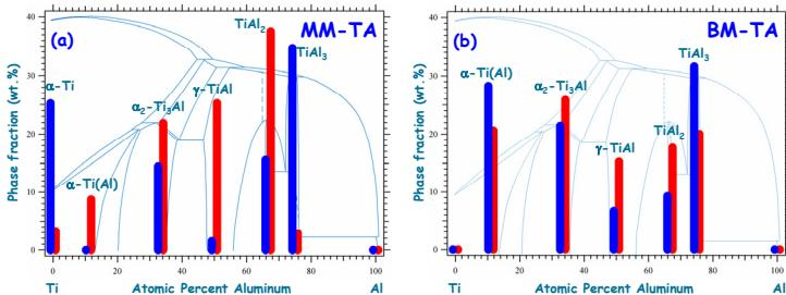
a and b: Phase fraction histograms before (blue) and after (red) the heating cycle as a function of Al concentration for MM-TA and BM-TA, respectively.
