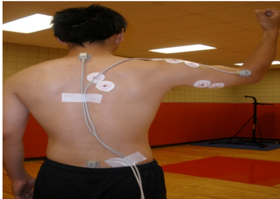
Figure 1. Example of electromagnetic sensor attachment.
