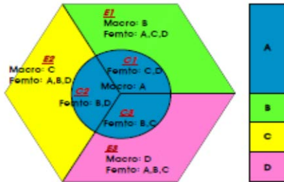
Figure 3: shows interference management approach using FFR
