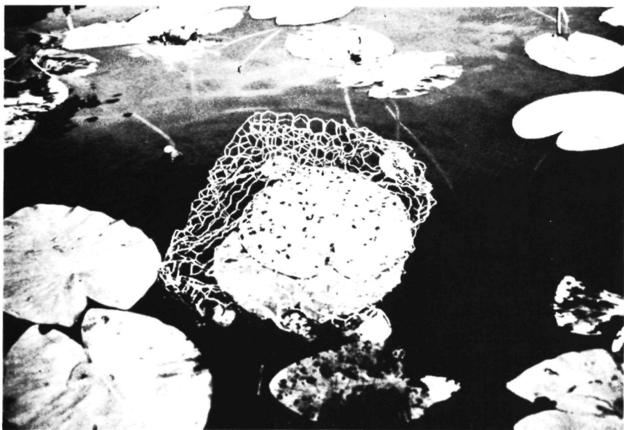
Fig. 2. Lime-trap for insects. For explanation, see text. The wire netting is kept floating by corks and is attached with a string to the petiole.
