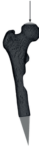
Figure 1. Anterior view of the FE-model, generated from a QCT scan. Displacement was applied to the model via the cup on the head of the femur, while the bottom of the model was fixated by means of high stiffness springs.
