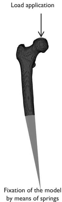
Figure 1. Boundary conditions for the FE model. The model was distally fixed by springs with a very high stiffness and the load was applied by means of a cup on the head of the femur, which incrementally displaced in distal direction.
