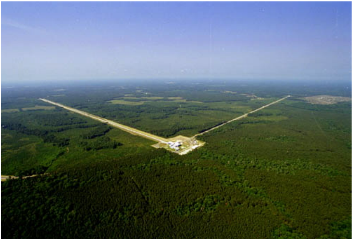
FIGURE 1.4: One of the several ground-based GW detector, namely the LIGO detector in Livingston, USA, with an armlength of 4 km. The other existing terrestrial detectors are: a second LIGO detector in Hanford, USA; Virgo in Italy; GEO in Germany; and KAGRA, which is being built in Japan.
