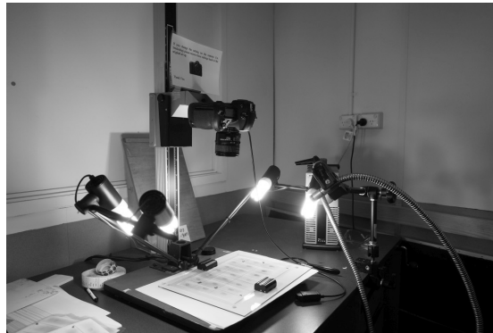
Figure 2.14: The operational Victoria Police Forensic Services camera setup that has been used for capturing pseudo fingermark images.
