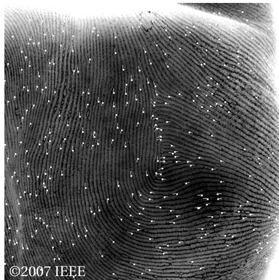
Figure 2.12: Adult ballprint image after extraction and minutiae detection, showing 352 minutiae. Published by Uhl and Wild [144].
