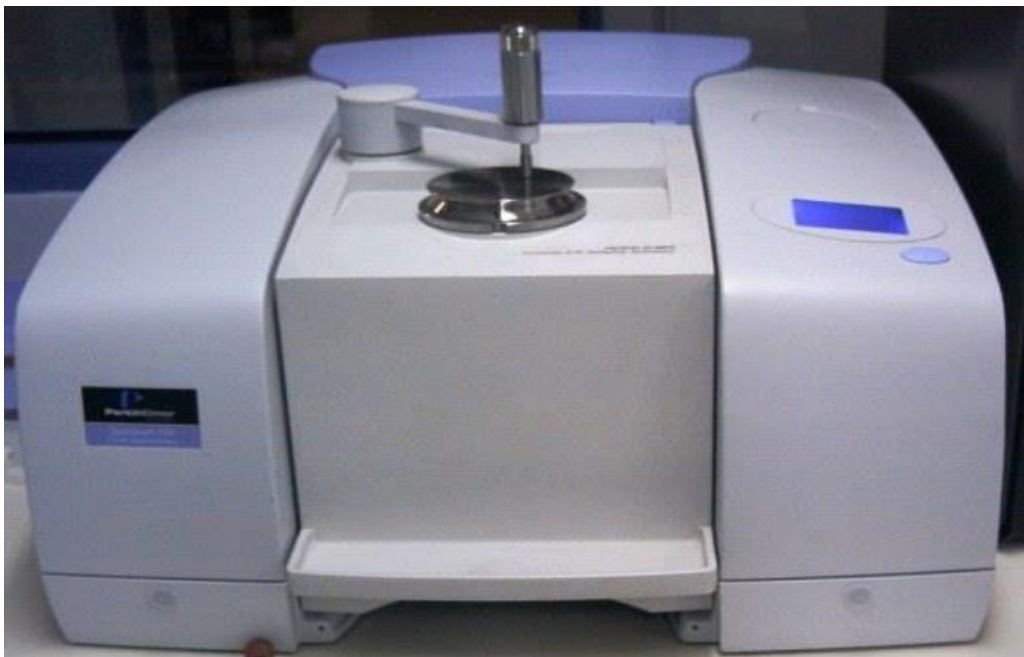
Figure 2.8 FTIR Spectrum 100 from Perkin Elmer (Antolasic, 2014).
