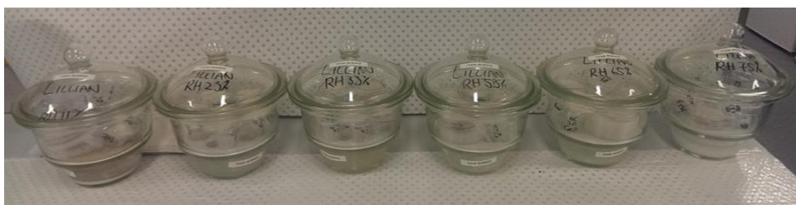
Figure 2.13 Series of relative humidity chambers (RH11% to RH75%) made with DURAN glass desiccators.
