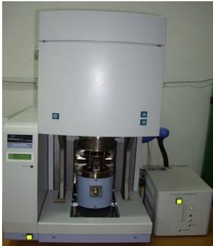
Figure 2.6 Diamond DMA from Perkin Elmer (Perkin Elmer, 2003).
