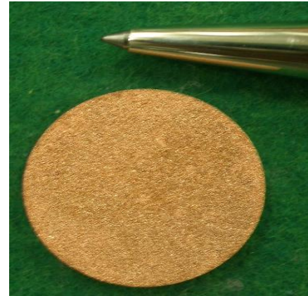
(c) Biporous layer as an evaporating face of the combined wick
