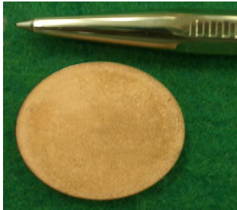
(b) Monoporous layer as an absorbing face of the combined wick
