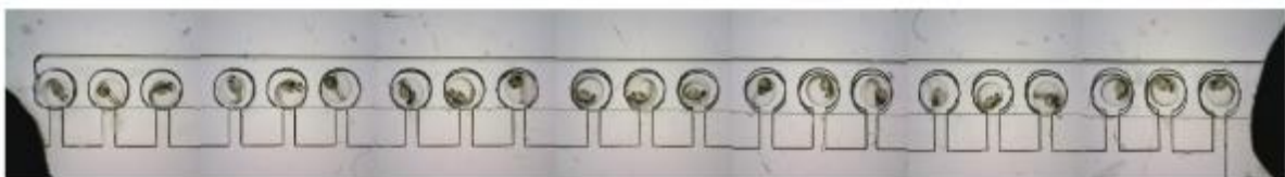
Figure 5.4.2 Bright field image from miniaturised Dino-Lite 5 MP USB microscope. Images of embryos were taken at a group of three and then stitched together and shown as an image of the whole chip.
