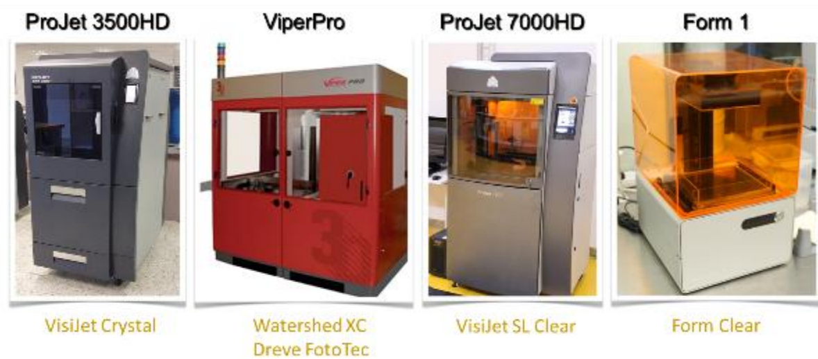
Figure 2.4.2 3D printers used in this study. From left to right: ProJet 3500HD is a MJM 3D printer using VisiJet Crystal material together with VisiJet S300 support wax. ViperPro is a SLA 3D printer using Watershed 11122XC resin or Dreve FotoTec Clear resin. ProJet 7000HD is also a SLA 3D printer using VisiJet SL Clear resin. And Form 1 is a SLA 3D printer as well using Form Clear resin. All the printing materials are specifically used for only their designated 3D printers.
