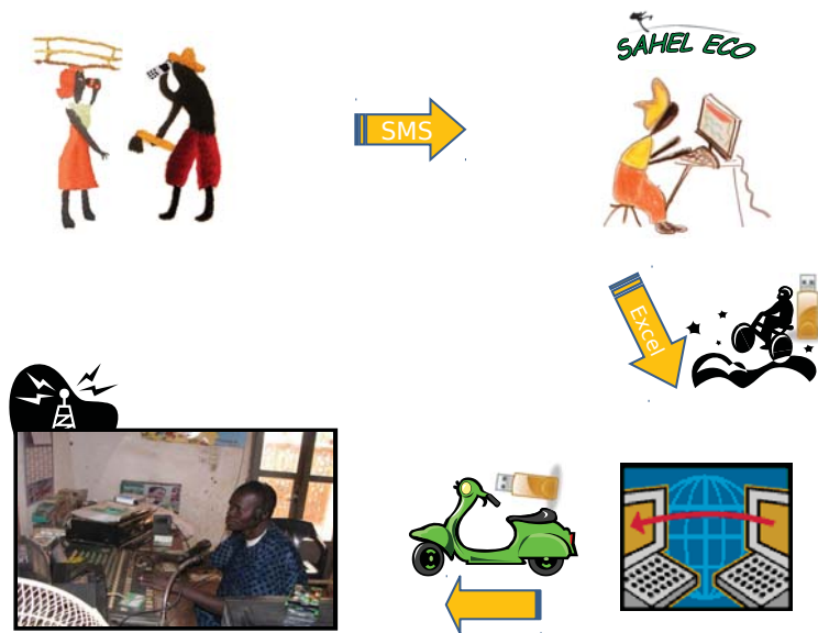
Figure 4.1: The original market information distribution infrastructure for rural farmers in the Tominian and Ségou regions of Mali. This diagram shows how information from the farm goes to the local radio station for broadcast to potential buyers. Credit: Sahel Eco & Anna Bon.
