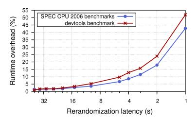
Figure 3.6: Run-time overhead against periodic rerandomization latency.
