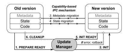
Figure 2.4: The state transfer process.
