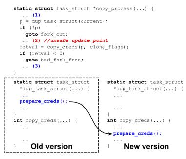
Figure 2.1: An unsafe live update using function quiescence.
