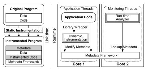
Figure 4.1: The RCORE architecture.
