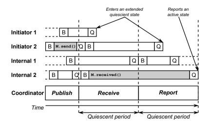
Figure 7.3: A sample run of our quiescence detection protocol.
