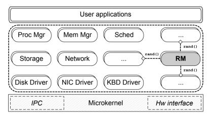
Figure 3.1: The OS architecture for our ASR design.
