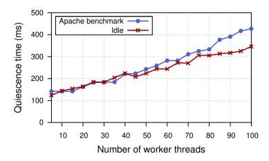
Figure 7.5: Quiescence time vs. number of worker threads.
