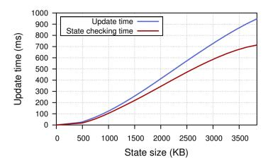
Figure 2.6: Update time vs. run-time state size.
