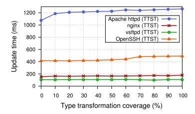
Figure 6.5: Update time vs. type transformation coverage.
