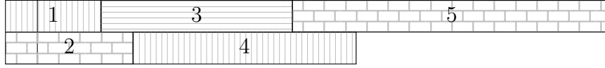
Figure 1.2: Gantt chart depicting the optimal schedule for minimizing the sum of completion times.
