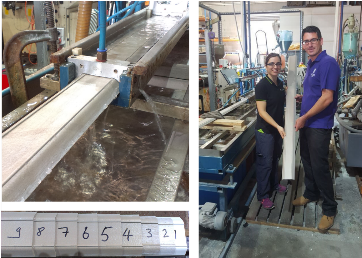
Figure 5.17: First biocomposite profiles extruded in an Australian industry
