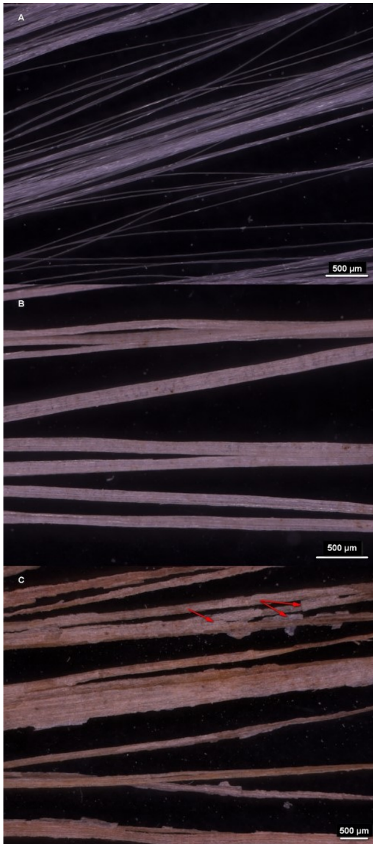
Figure 4.4: Optical microscope images of A) BioMid ® , B) Kenaf and C) Flax fibre samples (Images obtained with an Axio Zoom.V16 microscope by CIC).
