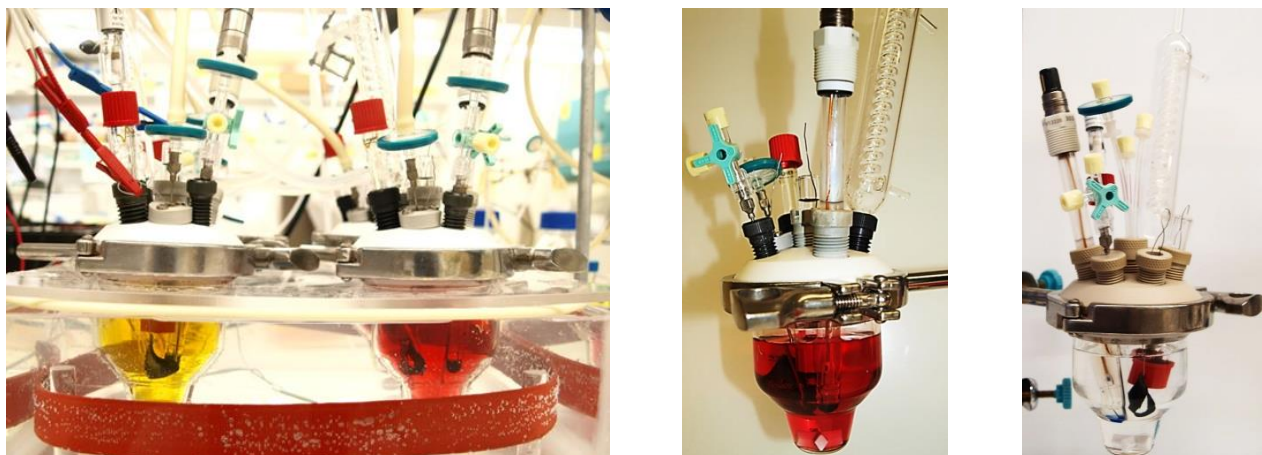
Figure 17: Pictures of the first (left and middle) and second generation (right) of bio-electrochemical system developed by CEMES. The system is suitable for anaerobic cathodic and anodic fermentations including electrochemical characterisation, controlling temperature, stirring, pH, reactor atmosphere and a three electrode setup connected to a potentiostat.
